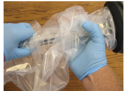
9. Squeeze middle of liner in left hand. Compress top end with right hand
