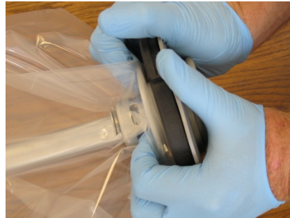
5. Squeeze fitment over o'ring
