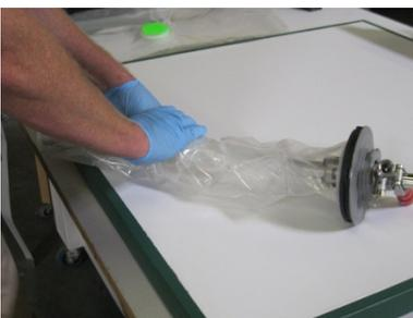
1. Never wrap the liner around the spear. This will restrict the liner from opening.
