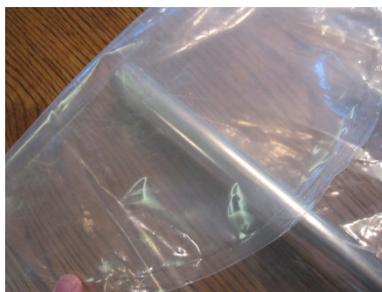
2. Make sure the spear is positioned at the base of the liner to avoid a liner fold as shown.
