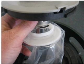
2. Lift handle & disengage liner fitment
