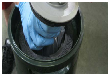
11. Clear liner from opening to avoid pinching liner
