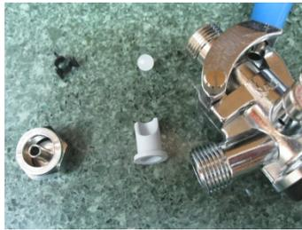
2. Remove check valve & ball lock
