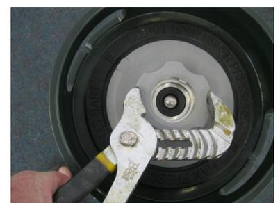
3. Never use a tool to remove the handle. Any pressure remaining in the keg will prevent handle from rotating. Always depressurize before removal.
